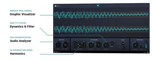
MIYA's real-time visualizer provides immediate feedback using four different colors. Short orange vertical lines indicate detected zero-crosses, while a grey line shows the incoming original signal. A blue line plots the generated signal, and a green line visualizes the output from the plugin, a mix of wet and dry signals.
